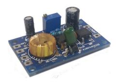
This PCB allows full control over the light levels of the attached lamps and LEDs. There are solder pads attached to this PCB so wiring up is quite straight forward.
